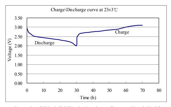
Discharge condition: under  $4.3k\Omega$  load till 2.0V end-point voltage; Charge condition: 3.1V of Constant Voltage,  $510\Omega$  of Protective resistance, charge for 40h.
