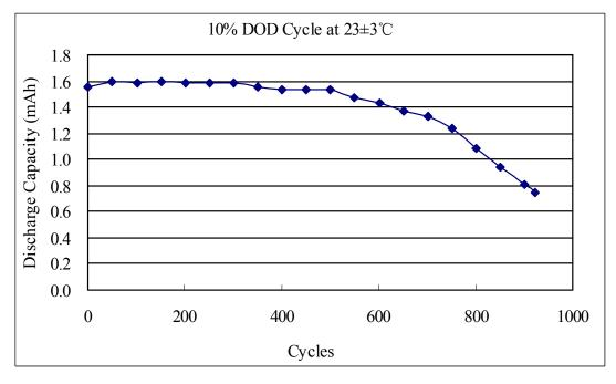
Discharge condition: under  $4.3k\Omega$  load dicharging 2.5h; Charge condition: 3.1V of Constant Voltage,  $200\Omega$  of Protective resistance, charge for 4h.
