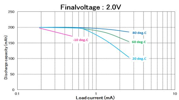
\* Nominal capacity indicates duration until the voltage drops down to 2.0V when discharged at a nominal discharge current at 20 deg. C.
